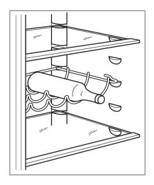
This bottle holder shelf can be tilted in order to store previously opened bottles. To obtain this result, pull the shelf up so it can rotate upwards and be placed on the next higher level.
